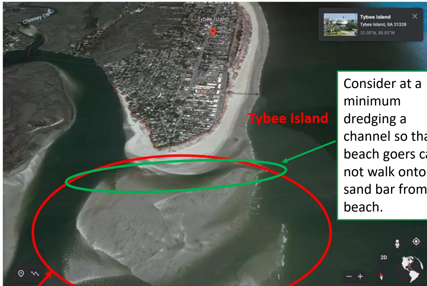
The ebb tidal delta, an accumulation of sand as a result of the north-south longshore transport, sits at the south end of Tybee Island. Google Earth
